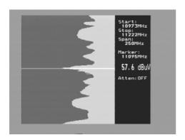
Rotate the LNB so that either the Horisontal or Vertical polarisation will be in its max-position –adjusting the **cross-polarisation**.
